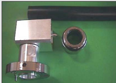
1) Flush cut the cable squarely.
