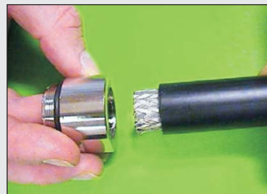
4) Slide the back section of the connector over the braid without disturbing it. Be sure that the axis of the connector is in line with the axis of the cable.
