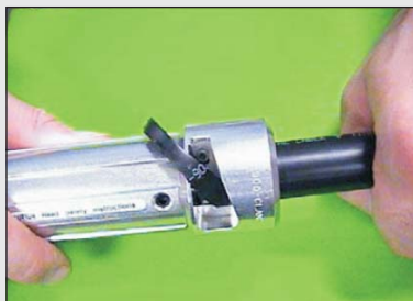
3) Strip the cable end using the ST-900/1200C prep/strip tool by inserting the cable into the proper end of the tool. (Be sure there is no jacket material stuck in the tool before beginning this operation.)
