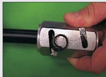
2) Strip the cable end using side 1 of the ST-600 clamp tool.
