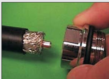
5) Make sure the braid is straight. Square the connector with the cable and twist onto the cable until it bottoms on the jacket.
