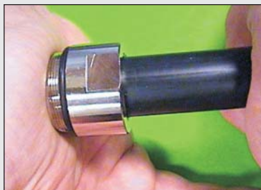
5) Use the palm of your hand to snap the back end of the connector over the jacket. Spinning the aff section in a clockwise motion while applying pressure will also help to properly position the connector.
