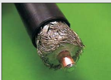
3) Deburr the center conductor using a file or deburring tool. All burrs must be removed.
