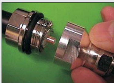
7) Begin threading the front of the connector onto the back end while keeping the back end firm against the jacket.
