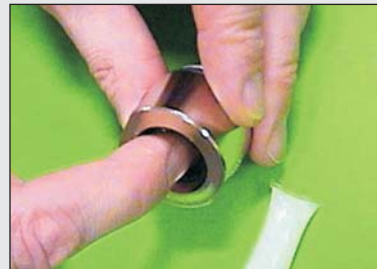
2) Cut the corner of the lubricant packet and apply the lubricant liberally to the O-ring in the aff section of the connector.
