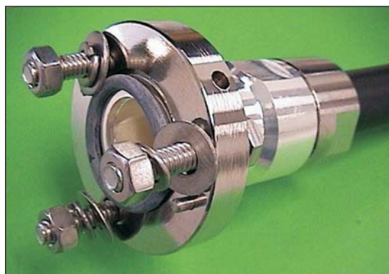
Figure 1 · The 7/8-inch EIA flange connector. For this application, the rubber O-ring is not required and will be removed prior to mating with the bulkhead.
