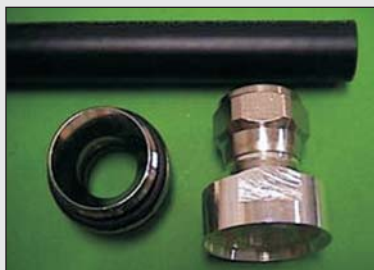
1) Flush cut the cable squarely.
