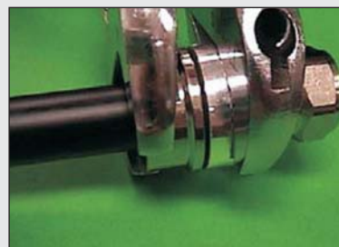
8) Tighten firmly using two 15/16" open end wrenches, or adjustable wrenches.
