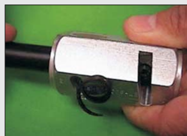
4) Strip the jacket using side 2 of the ST-600 clamp tool.
