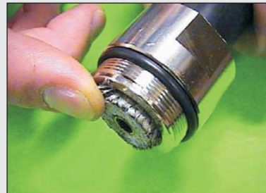
6) The braid should then be spread across the face of the connector.
